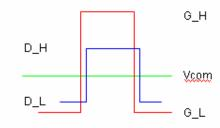
Ex. LC=5V, Vcom=0V Data H=+/-5V, Data L=0V, Data Gray=+/-3V Gate H=-6~+18V, Gate L=-6V Just suggestion!
